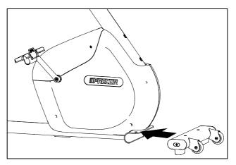
Figure 4: Front stabilizer installation
